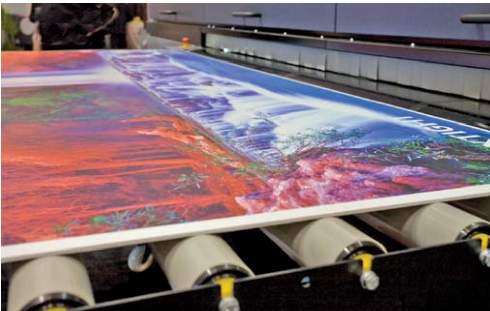
Fig. 3: Many UV printers can image 4 x 8-ft. boards. Usually the pieces are fed from the 4-ft. side. Notice that the Rho 800 can handle the long, 8-ft. side.
